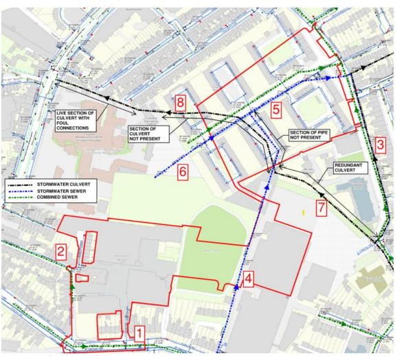
Figure 2-1: Reference Plan of Existing Sewers - IW Record Map Extract
