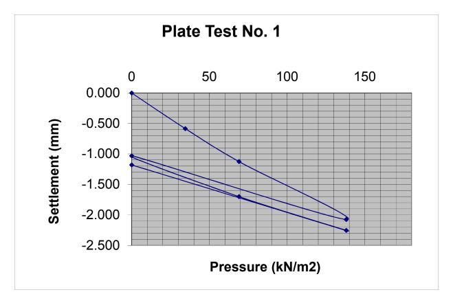
Modulus of subgrade reaction, K (Initial) = 41.44 MN/m2/m
